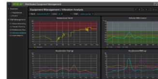
Facility 3-axis vibration detection
